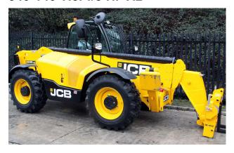
Max lift capacity **4,000kg**Max lift height **13,780mm**Max forward reach **9,640mm**Capacity at maximum reach **1,250kg**Engine power gross **75hp(55kW)**
